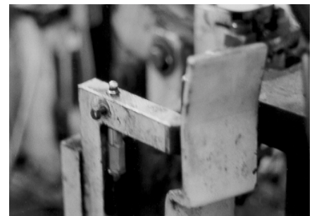
Figure 3. The sensor at left was repeatedly damaged until it was placed into a SoftNoze Banking Screw Adapter (right) that isolated it from damage.
