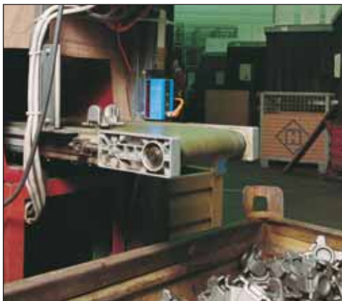
Fig. 4 Counts irregularly shaped objects during production
