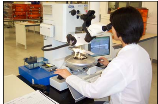
Destructive testing to ensure wire bond quality
