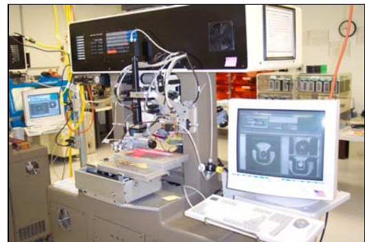
High speed automated die attach
