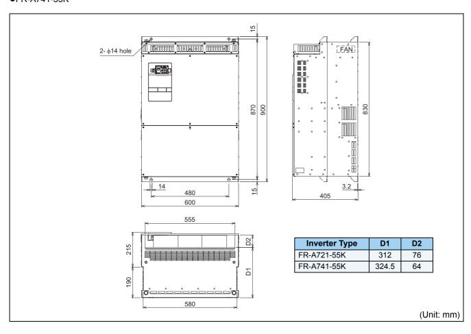
When encasing the inverter in an enclosure, the generated heat amount in an enclosure can be greatly reduced by installing the heatsink portion of the inverter outside the enclosure.
